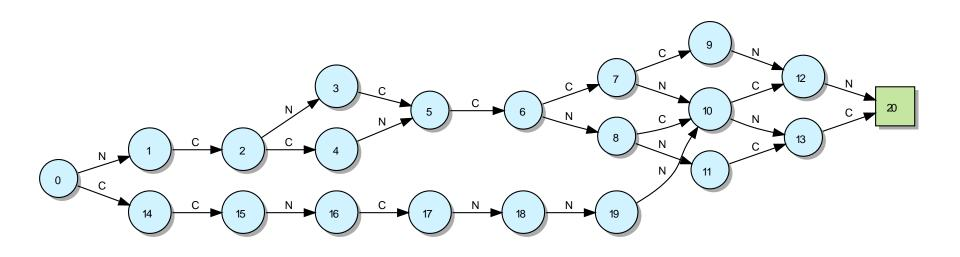
Simultaneously matching all 14 imidazotriazine SMARTS can be accomplished by the above finite state machine (FSM). A single SMARTS match is conceptually a linear state sequence.
